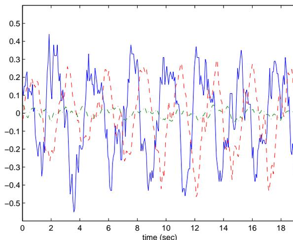
Figure 4.12: A plot of the feedback the policy acquired during simulation run 3 applied to the robot vs. the lateral tilt and linear velocity. The blue, solid line shows the absolute feedback applied. The red, dashed plot is the lateral linear velocity of the upper body and the green dash-dotted line represents the lateral tilt.
