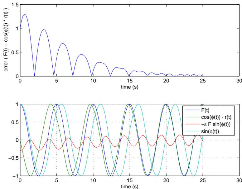
Figure 2.4: The evolution of a simple, perturbed Hopf oscillator.  $\epsilon = 0.3$ ;  $\mu = 1$ ;  $\phi_o = \frac{\pi}{2}$ ;  $\omega = \omega_e = 0.2 \cdot 2\pi$ . The upper plot depicts the error between the force and the output of the oscillator. The lower plot shows the force  $F(t)$ , the output of the oscillator  $\cos(\phi(t)) - r(t)$ , the coupling  $-\epsilon \cdot F \cdot \sin(\phi(t))$  acting on the phase velocity and  $\sin(\phi(t))$ .
