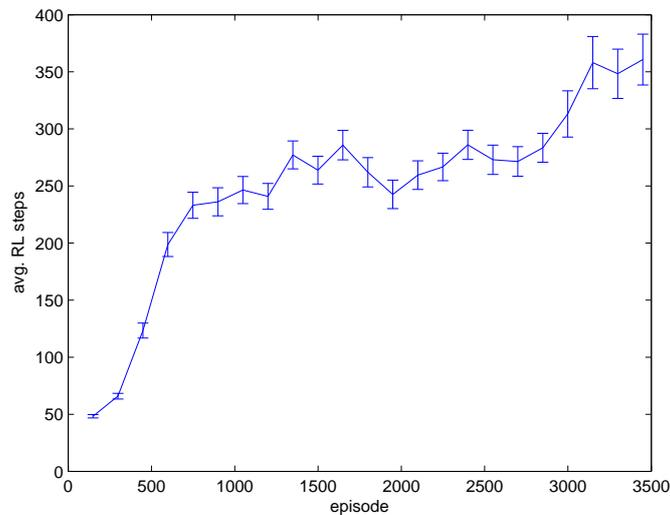
Figure 4.6: The Extra-tree based batch mode algorithm with a four dimensional state vector and a Webots time-step of 1ms running for 3540 episodes. The error bars show the standard error of the number of steps per episode averaged over 150 episodes.
