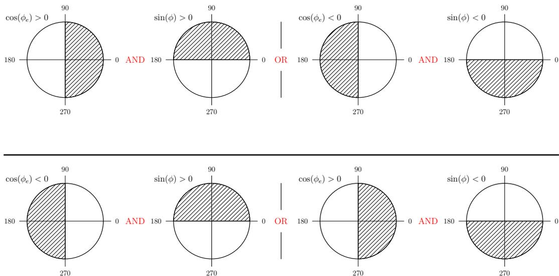
Figure 2.3: The upper part of the figure shows the conditions to be satisfied by the systems in order to decrease the phase velocity. The lower part shows the conditions for increasing the velocity.
