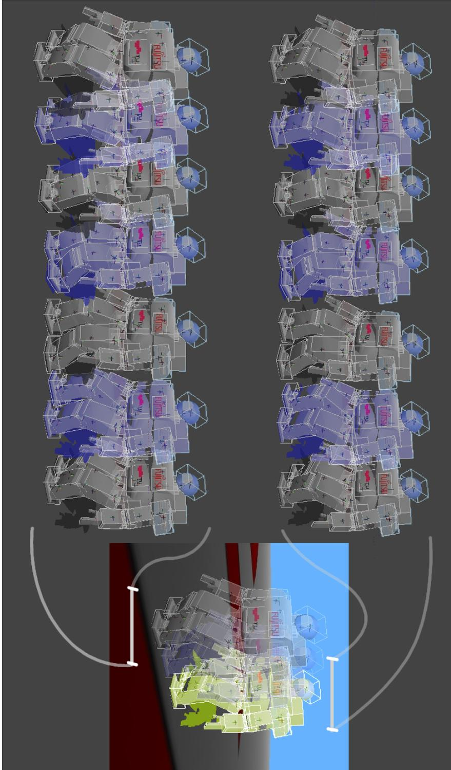
Figure 4.13: Walking gait of the Hap-2 robot during an episode of run 2. The frames are evenly spaced. The distance the robot moves from one frame to the next is therefore linearly related to the distance moved in the simulation.
