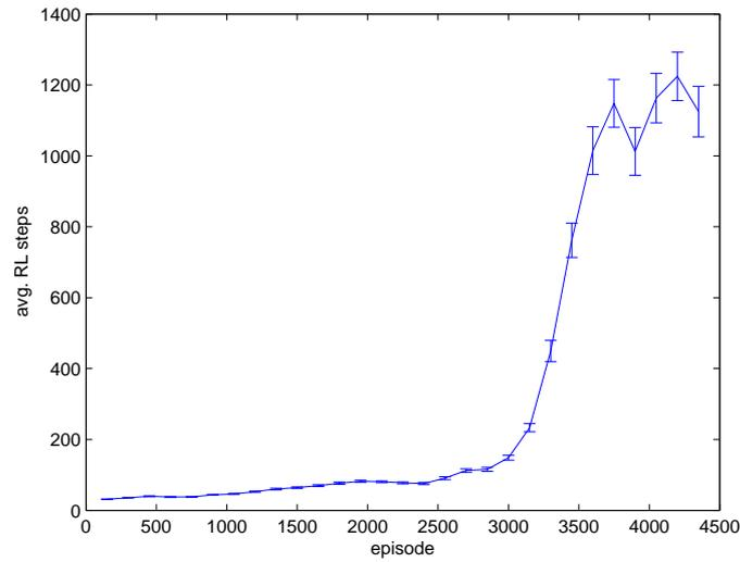
Figure 4.7: The SARSA( $\lambda$ ) algorithm with a three dimensional state vector and a Webots time step of 8ms running for 4542 episodes. The error bars show the standard error of the number of steps per episode averaged over 150 episodes.
