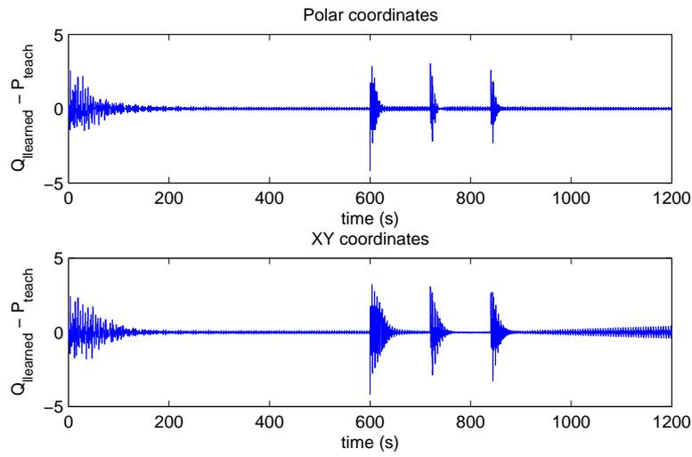
Figure 2.6: Error plot of a PCPG learning a periodic input signal and later during several perturbances. The upper plot is the version in polar coordinates with the improvements discussed in the text added to it, while the lower graph is the system as published in [Righetti et al. 2005]. The perturbations were applied to all but the first oscillator, in order to make plotting the error easier.
