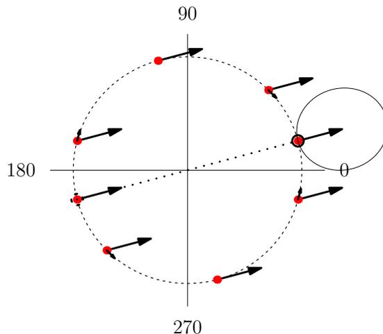
Figure 2.2: The phase point of the autonomous oscillator in a polar reference frame rotating with  $\omega_e$ . The phase point has a stable (marked with a circle) as well as an unstable equilibrium point (marked with a dashed circle). The big arrows denote the average direction of the external force, whereas the smaller arrows indicate the direction on the limit cycle in which the phase point is dragged by the force.
