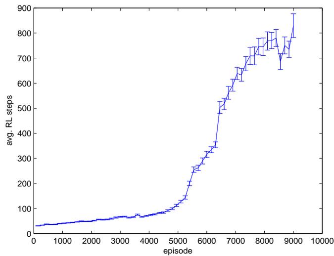
Figure 4.5: The SARSA( $\lambda$ ) algorithm with a four dimensional state vector and a Webots time-step of 1ms running for 9052 episodes. The error bars show the standard error of the number of steps per episode averaged over 150 episodes.
