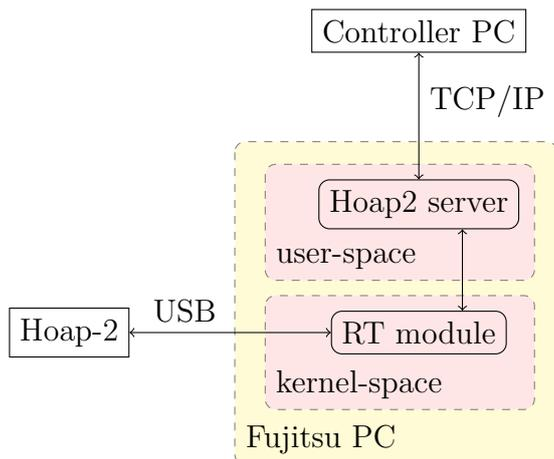
Figure 4.1: The architecture of the Hoap-2 interface software.
