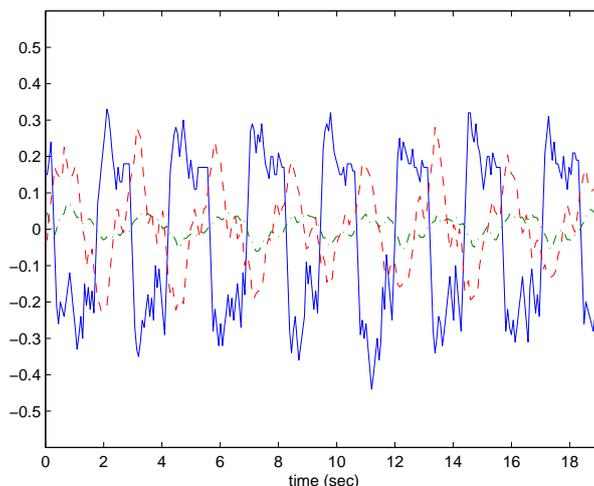
Figure 4.11: A plot of the feedback the policy acquired during simulation run 2 applied to the robot vs. the lateral tilt and linear velocity. The blue, solid line shows the absolute feedback applied. The red, dashed plot is the lateral linear velocity of the upper body and the green dash-dotted line represents the lateral tilt.
