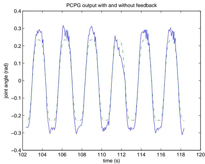
Figure 4.8: The output of the first PCPG without any feedback (green dash-dotted) and with the radius feedback applied (blue) during an episode of run 1.
