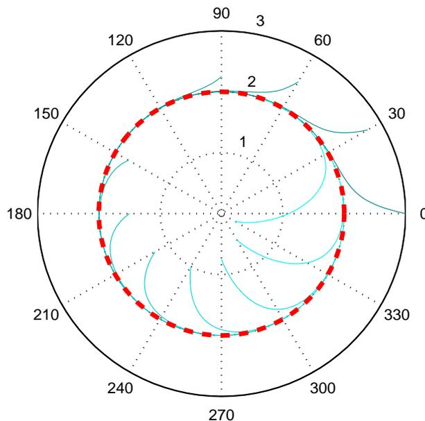
Figure 2.1: The limit cycle (red, dashed) of a simple Hopf oscillator with  $\mu = 4$ ;  $\omega = 0.2 \cdot 2\pi$  and a few evolutions of the system with varying initial conditions in a phase plot ( $\phi$  plotted against  $r$ ).
