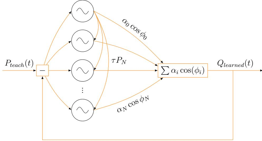
Figure 2.5: The structure of a network of coupled oscillators representing a PCPG. The term  $P_i$  is defined as  $P_i = \sin(R_i - \phi_{i,\Delta} - \phi_i)$  for layout reasons. Adjusted from [Righetti et al. 2005].
