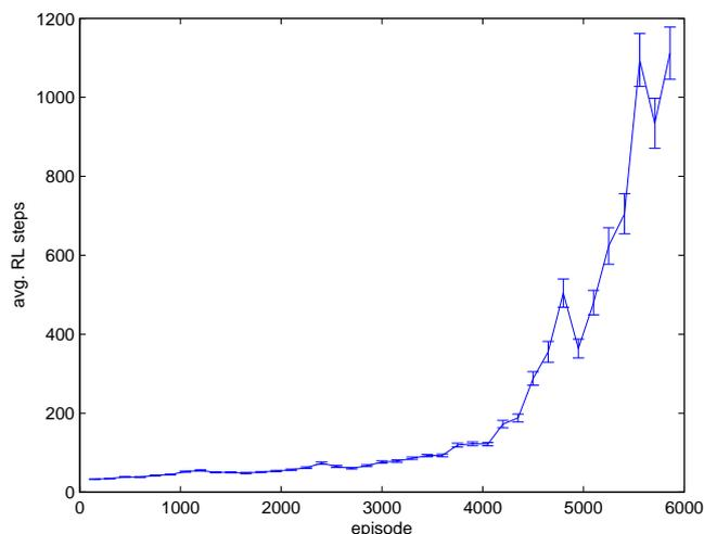
Figure 4.4: The SARSA( $\lambda$ ) algorithm with a three dimensional state vector and a Webots time-step of 1ms running for 5935 episodes. The error bars show the standard error of the number of steps per episode averaged over 150 episodes.
