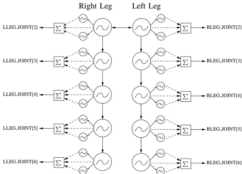
Figure 4.2: The structure of the PCPG system. Taken from [Righetti and Ijspeert 2006].
