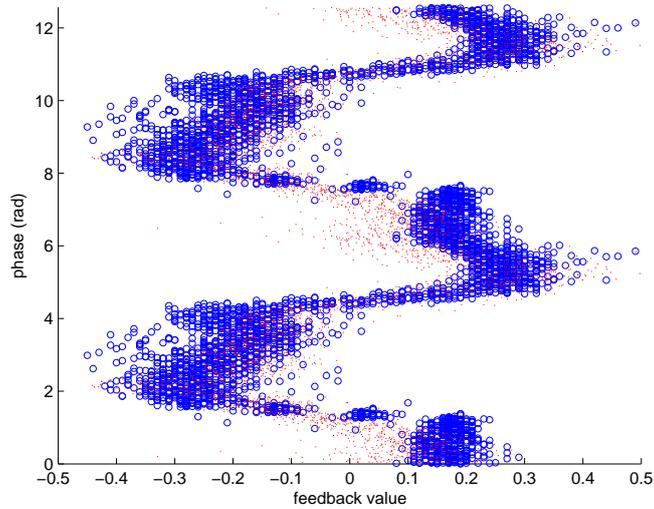
Figure 4.9: A scatter plot of the phase vs. the absolute feedback during an episode of run 2. The blue dots are the feedback as learnt by the RL agent, while the red dots represent a linear model of the feedback.
